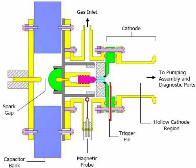
Figure 1. Schematic of the pulsed capillary discharge.
