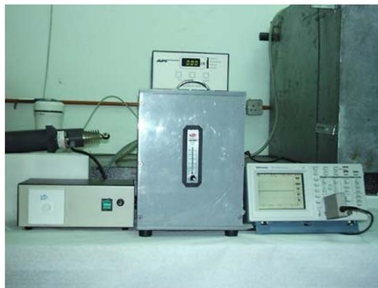
Fig. 5 An ozonizer unit based on the DBD.
