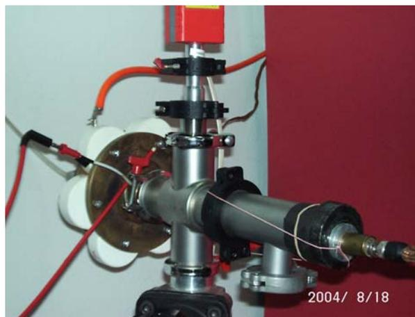
Fig. 3. The pulsed capillary discharge.
